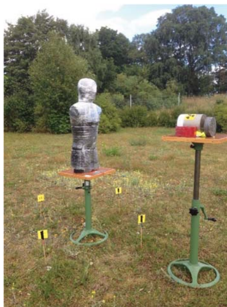
Figure 6. Experimental set-up at the exposure site. The table on which the phantom was positioned allowed the phantom to be rotated while the radiation source was fixed in one position
