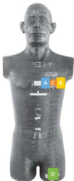
Figure 5. Position of the TLD- and OSLD holders outside the phantom: A.) TLD holder for measuring personal dose; B.) same TLD holder as (A) but with NaCl for OSL read-out; C.) new version of OSLD holder with salt; D.) ordinary salt package found in restaurants. N.B. in the image the phantom is not covered in plastic foil.
