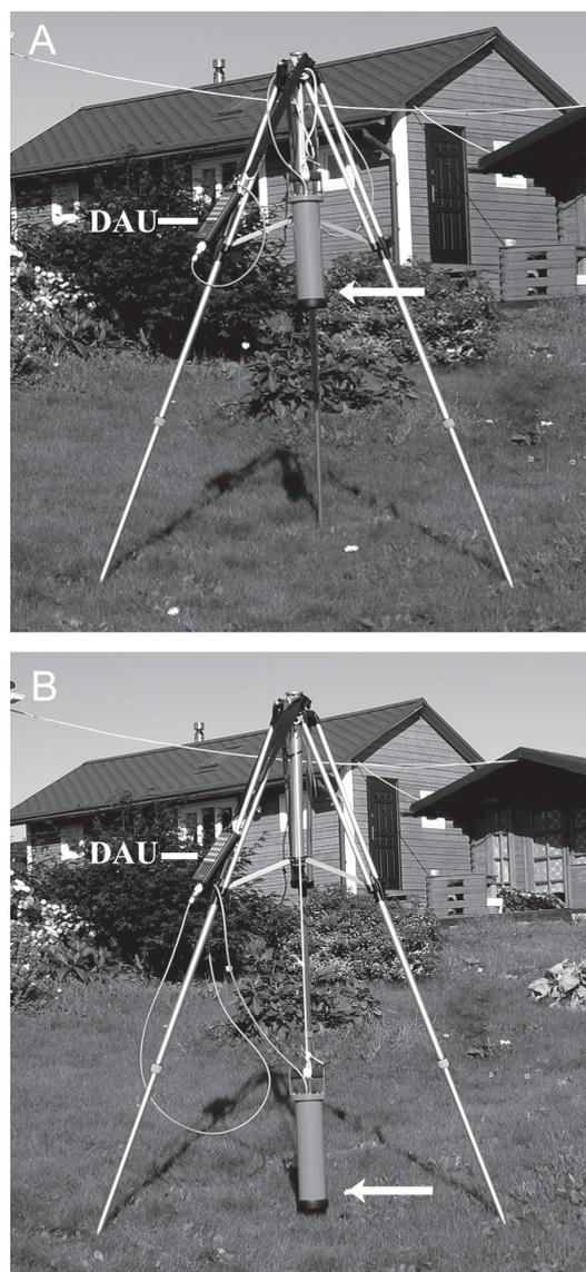
**Fig. 1.** *In situ* gamma-ray spectroscopic measurements with MKS AT6101D at a kitchengarden in Khittolovo (plot Hit-2), the Leningradskaya region in 2015. The detection unit and the data analysis unit (DAU) are set up on an aluminum tripod. The white arrows indicate approximate position of the effective center of the detector: at a height of about 1 m (the top panel A) and 0.1 m (the lower panel B) above the ground
